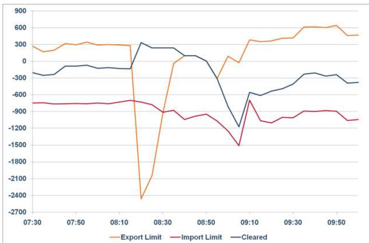
Figure 9 MW Flow and Limits of Victoria to NSW Interconnector
