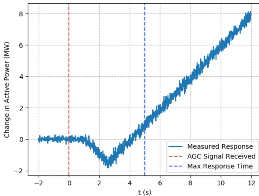
Figure 3 is an unacceptable response because there is a negative drift in power output, and while the ramp does commence before 5 seconds, the output at  $t=5s$  is still below the original basepoint output.
