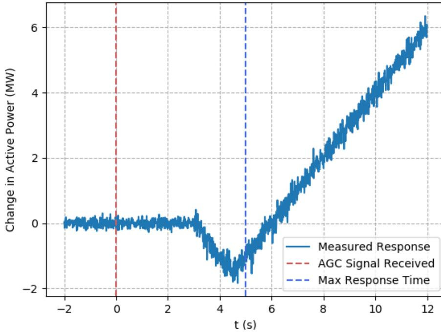
Figure 4 is an unacceptable response because the high level of noise obscures the commencement of the ramp and it is ambiguously close to the 5 second response time limit.
