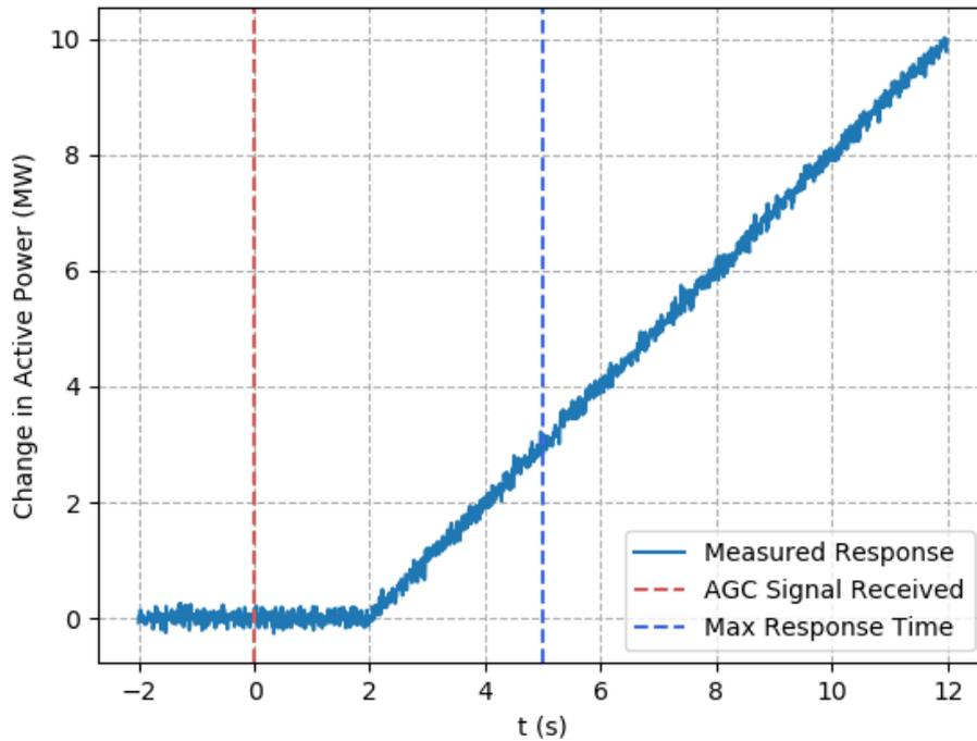
A deviation from the original basepoint is acceptable provided that the unit begins ramping within 5 seconds and the change in active power ( $\Delta P$ ) at  $t=5s$  is positive. Figure 2 shows an acceptable response despite the negative drift before starting the ramp.
