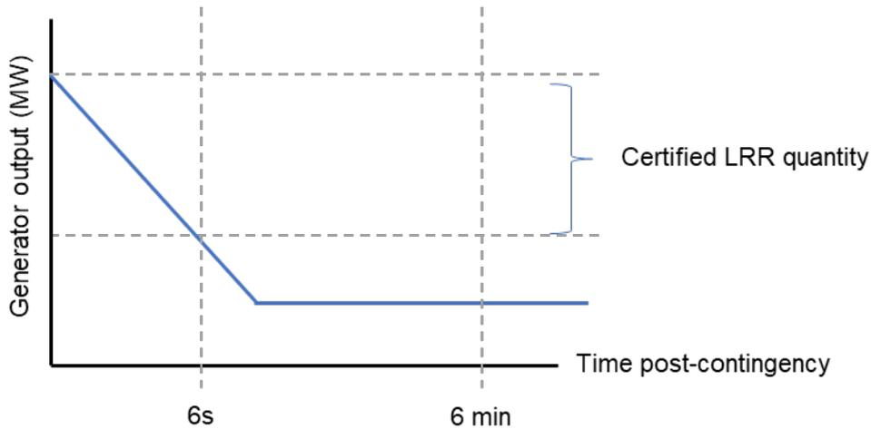
Figure 12 Fast ramp-rate and overshoot LRR response
