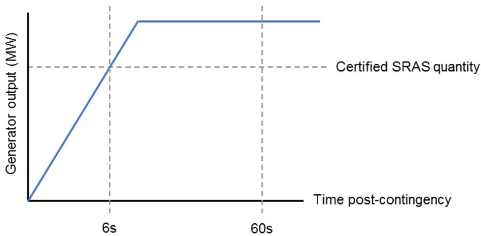
Figure 8 Fast ramp-rate and overshoot SRAS response
