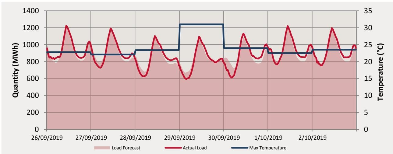
The maximum temperatures for this trading week ranged from 22.1°C to 31°C. The actual load peaked at 1224.327 MWh on the 26/9/2019.
